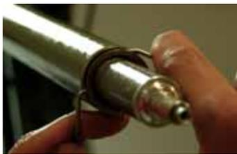
35. Grease the threads on the topcap assembly.
