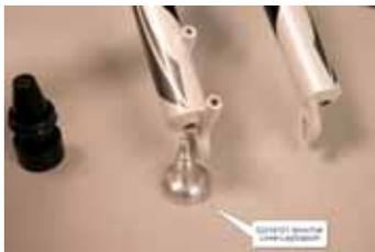
26. Insert the tool into the top of the lower leg, and then firmly strike the tool with a plastic mallet until the dust wiper is firmly seated into the lower leg.
