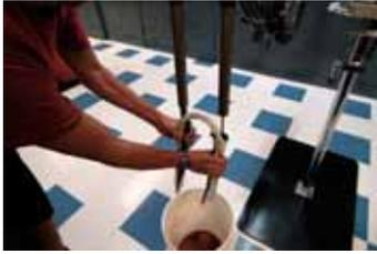
13. Using a 26mm socket wrench, remove the topcap. Lift the damper up slightly to expose the underside of the topcap assembly.
