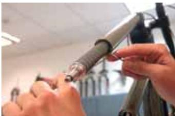
17. Carefully remove the cartridge through the bottom of the right upper tube.
