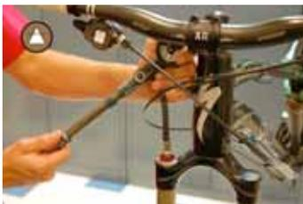
**Note:** Don't forget to slide the travel o-ring onto the left upper tube before continuing.
