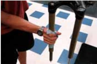
16. Use a pair of picks to remove the retaining clip on the bottom of the right upper tube. Use care not to scratch any exposed surfaces.
