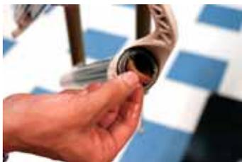
29. Use a shop towel to clean away suspension fluid from the dust wiper area. Leaving suspension fluid in this area can degrade the grease applied in the next step.
