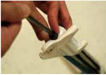
46. Screw the damper side bottom nut onto the damper cartridge.
