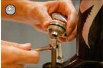
38. Tighten the topcap assembly with a 26mm socket wrench.
