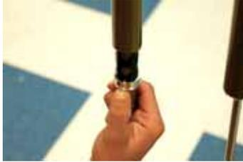
34. Use care and patience to install the clip back into the bottom of the right upper tube. Be careful not to scratch any surfaces with the pick. The second photo shows a profile of the clip; it's semi-coiled—a detail that may help in its insertion.
