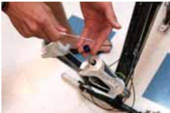
8. Use a 12mm socket and wrench to loosen the bottom nut bolt on both sides of the bottom of the fork. **Do not remove them just yet.**
