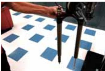
14. Using a 10mm open-end wrench, hold the damper shaft steady as you loosen and then remove the topcap with a 26mm socket wrench.
