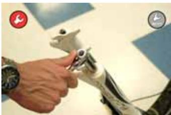
48. Install the compression knob onto the right side bottom nut. Use picks to install the circlip into the inside diameter of the knob.
