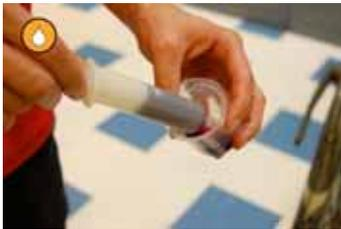
43. Place **10 mL** of suspension fluid in each leg. To access the lower leg hole on the dead side, use a hex key wrench to pull up on the dead side plunger. You can place the bottom nut onto the wrench beforehand to facilitate its installation.
