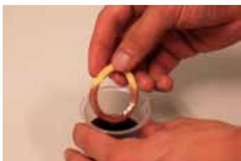
28. Insert both foam rings back into the lower leg assembly. To facilitate insertion, you might want to squeeze them into a "taco" and then slide them into their slot.
