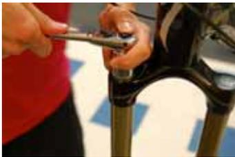
40. Use a high-pressure shock pump to inflate the damper cartridge just enough so the damper cartridge will hold its position as you slide the lower leg assembly on in the next step.
