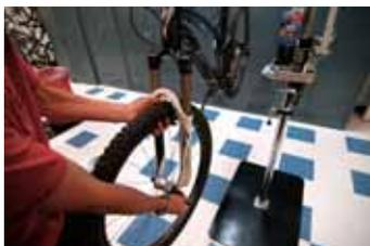
4. Clean the external surfaces of the fork with soap and warm water or isopropyl alcohol. Use a rag to dry the surfaces off.
