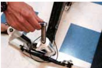
9. Make sure each bottom nut is threaded in at least 3 full turns from the top. Use a mallet to firmly tap the top of each bottom nut. This dislodges the cartridge and dead side device from the bottom of the lowers.
