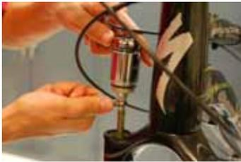
39. Torque the topcap assembly to **120Kgf-cm** using a torque wrench.
