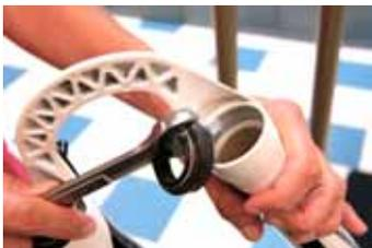
24. Place new dust wipers onto the dust wiper installation tool).
