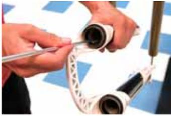
22. If you are re-using the foam rings, squeeze out the suspension fluid.
