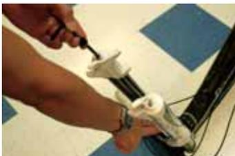
45. Slide the bottom nut down and screw the bottom nut while holding the hex wrench, to prevent the plunger from spinning.
