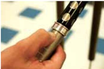
33. Slide the cartridge in through the bottom of the right fork leg while keeping the negative air spring setting with your finger. Once the majority of the cartridge has been pushed up through the upper tube, you can safely remove your finger from holding the negative air spring setting steady.
