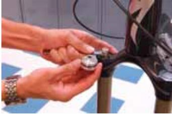
15. Use shop towels to clean the exposed upper tubes. Note the user's negative air spring setting. The default setting is 50mm , but could have been set differently during a previous service.
