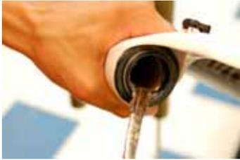
31. Grease all seals and threads on the cartridge.
