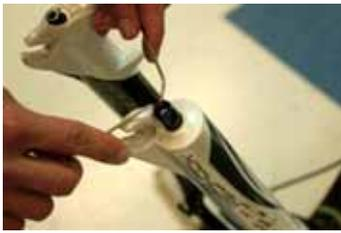
49. Place the plastic cap onto the compression knob.
