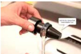
25. Insert the opening of the lower into the lower leg stabilizer tool. Insert the same side in which you're installing the dust wiper on.
