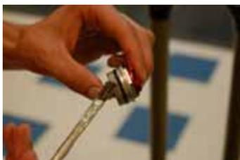
36. Using a 2mm hex wrench, turn the rebound adjuster screw in the shaft rebound insert until the two top surfaces are flush with each other, as shown.
