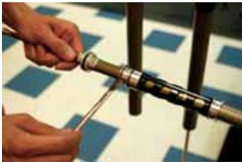
32. Set the negative air spring to 50mm, unless it has been set to a different user specification, as noted in step #16. Use your finger to keep the negative air spring setting in place as you maneuver the cartridge.
