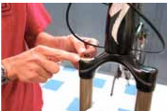
7. Turn the bike upside down to better access the bottom of the fork. Remove the rubber cap from the compression knob, then use a couple of picks to remove the circlip, which keeps the knob in place. This is a finicky clip, so take your time.
